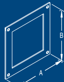
BOX FITTING Used when wireway enters an enclosure on the inside of the enclosure to provide a tight seal
